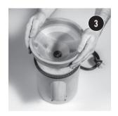
Take the hopper and turn it one full time clockwise. Then plug the mill into the power socket and switch on. Turn the mill further until you hear a slight ticking noise.
